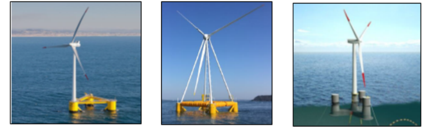
Figure 3: Semi-submersible examples: Windfloat (courtesy: Principle Power), Eolink (courtesy: Eolink) & OO Star (courtesy: Dr. techn. Olav Olsen)
