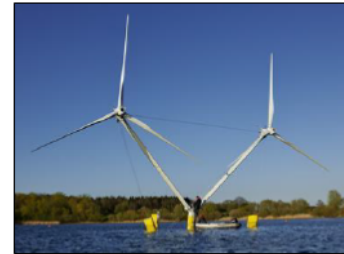
Figure 7: Multi-Turbine example: SCD Nezy2 (courtesy: Aerodyn)
