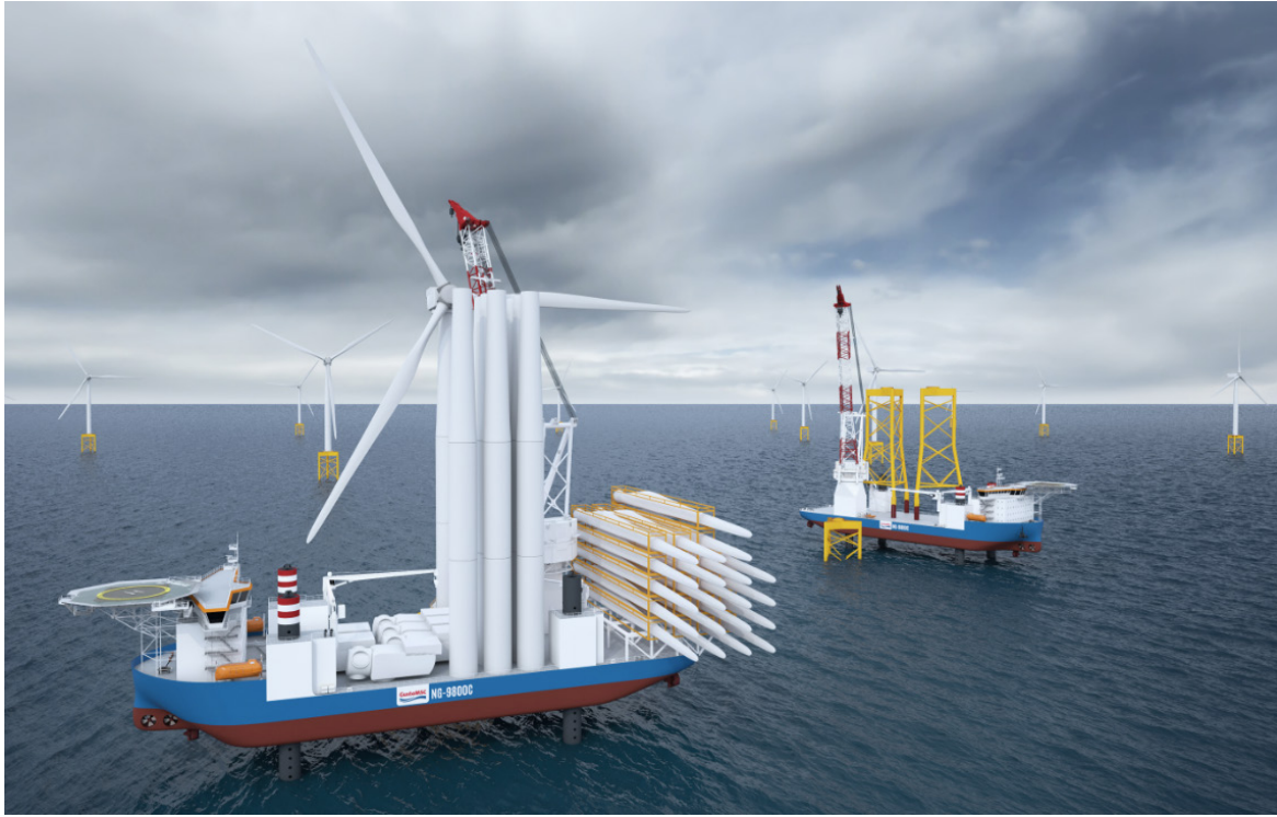
Figure 13. Rendering #4 of two NG-9800C-US installing turbines (left) and foundations (right)
