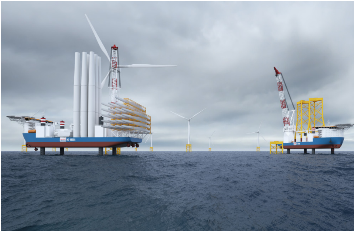
Figure 13. Rendering #4 of two NG-9800C-US installing turbines (left) and foundations (right)
